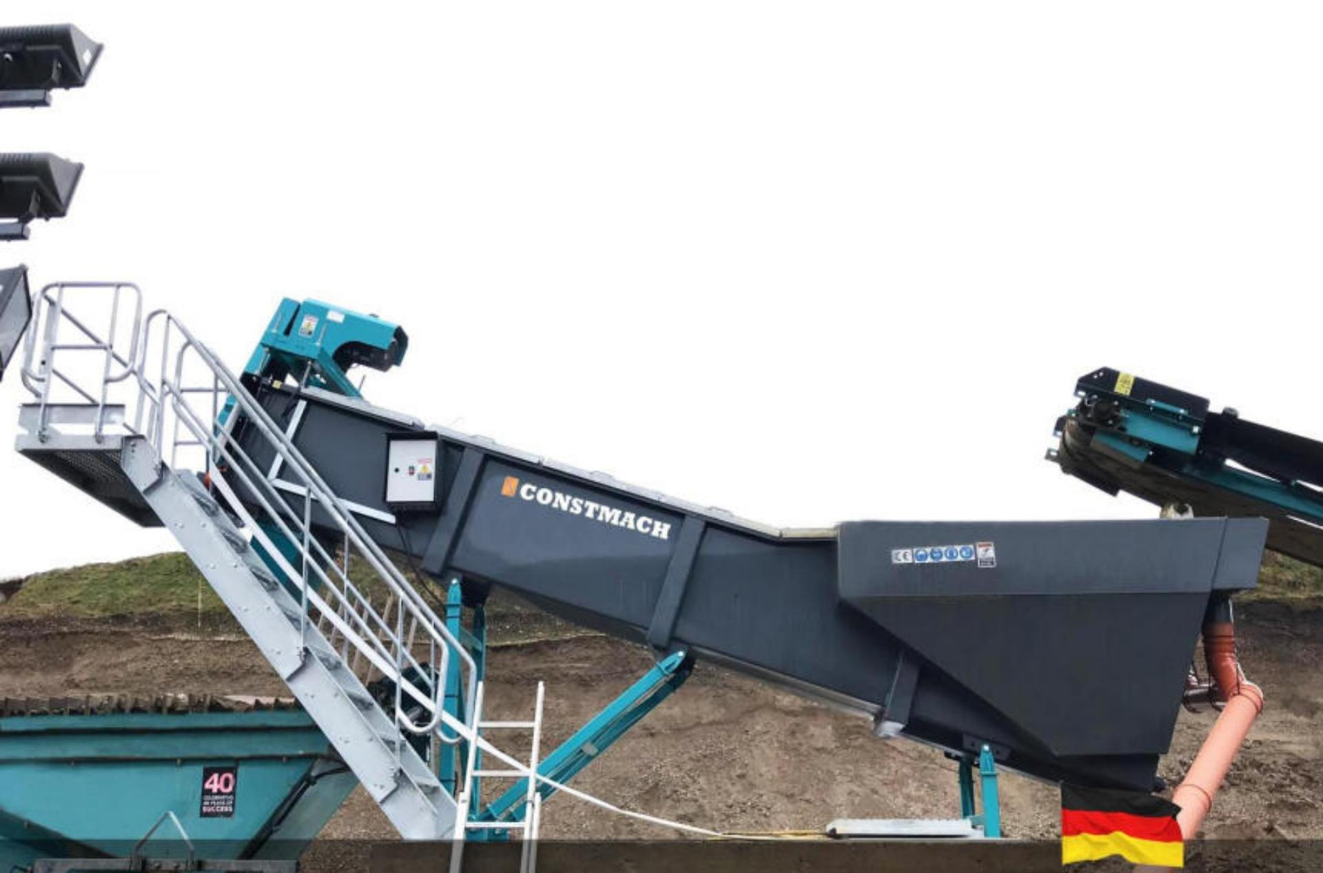
SW-7575 / PUŽNI DEHIDRATOR ZA PESAK
