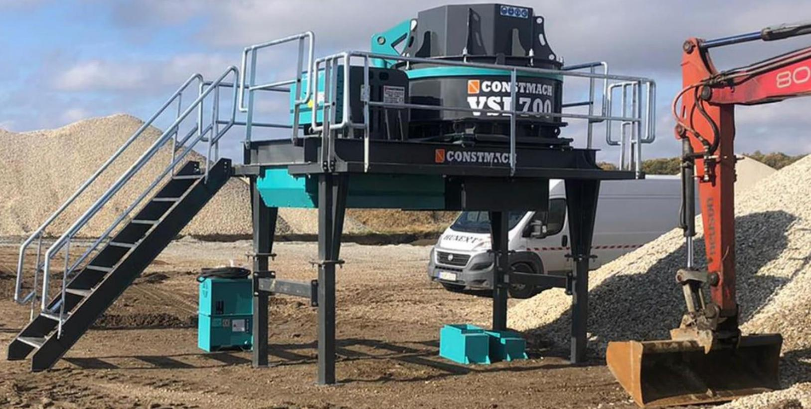
**VSI 700 CR / UDARNA DROBILICA SA VERTIKALNOM OSOVINOM**
