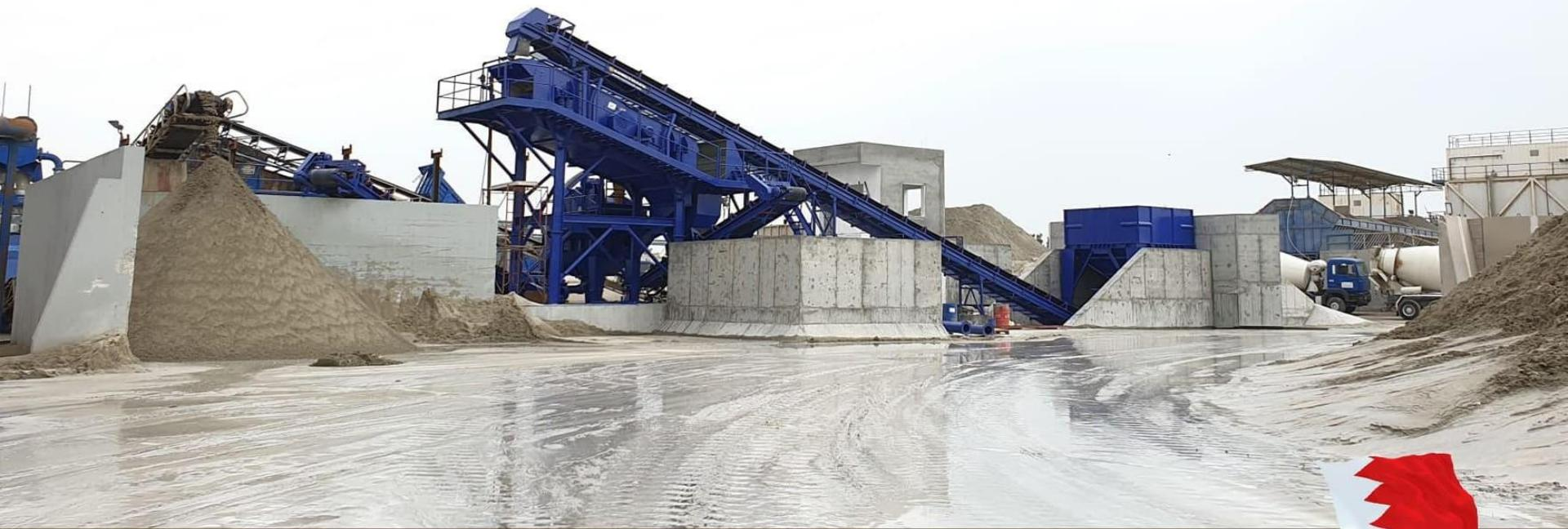
PUŽNI DEHIDRATOR ZA PESAK SA HIDROCIKLONOM
