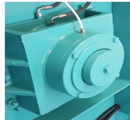
HIDRAULIČNI PAKET SA RUČNIM OTVARANJEM
