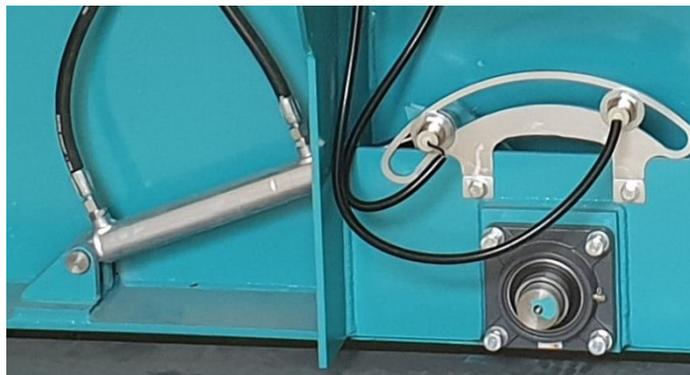
OTVOR ZA PRISTUP SA SIGURNOSNIM PREKIDAČEM
