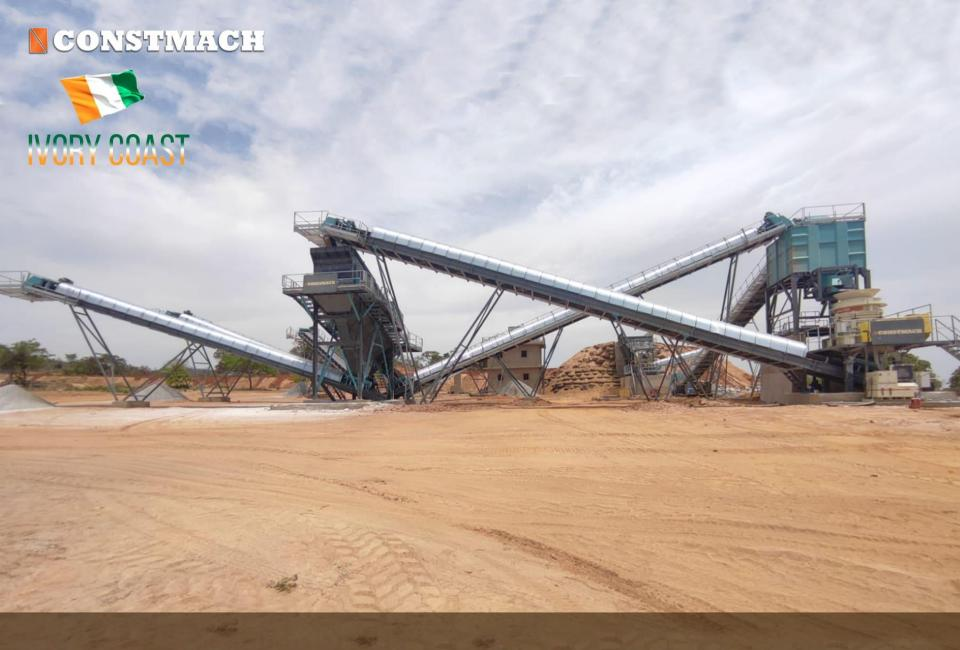
FIX JC - 3 / STATIONARY CRUSHING AND SCREENING PLANT
