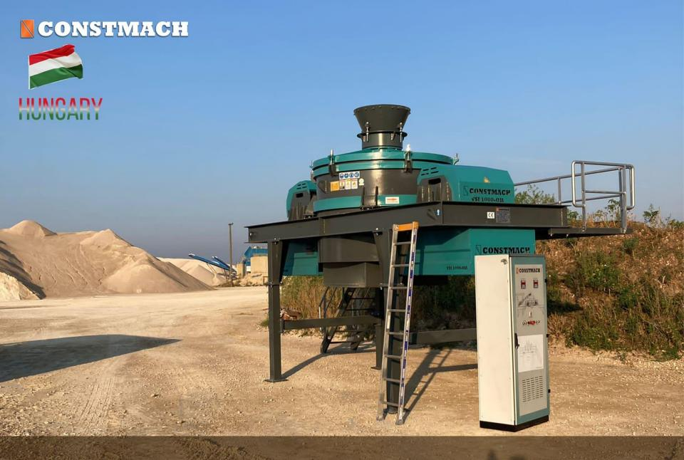
VSI 1000 / OPEN ROTOR VERTICAL SHAFT IMPACT CRUSHER
