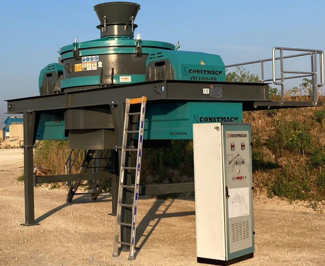
**VSI 1000 / OPEN ROTOR VERTICAL SHAFT IMPACT CRUSHER**
