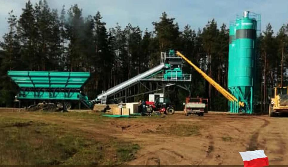
MOBILE 120 / CONCRETE BATCHING PLANT
