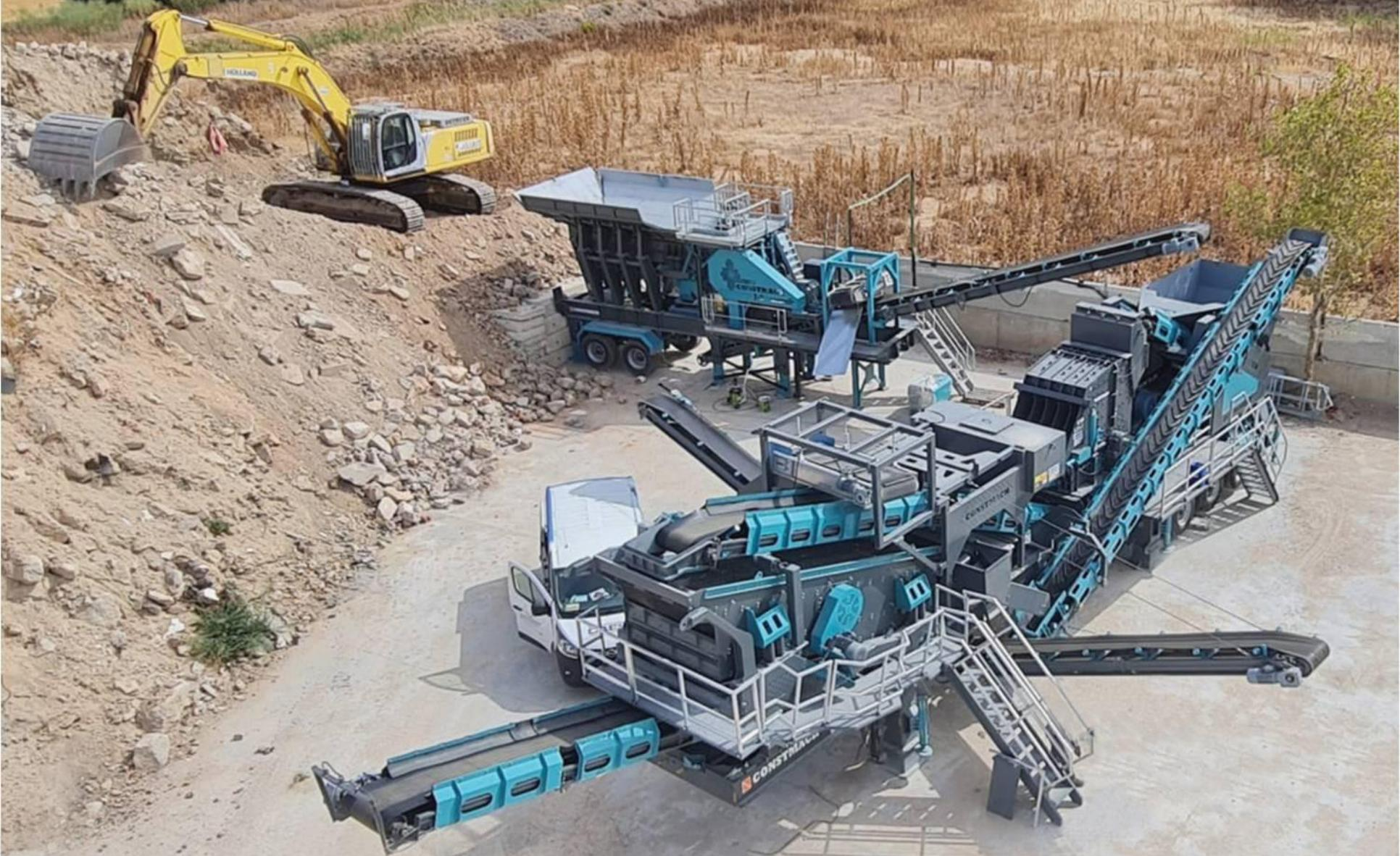
**CONSTMACH mobile jaw and impact crushing plants** are designed to crush a wide range of rock types, from limestone to basalt. The primary jaw crusher efficiently processes large and hard rocks, while the secondary impact crusher ensures the production of well-shaped, cubic final materials. Depending on customer requirements, the final output size can range from **0 to 60 mm**.
