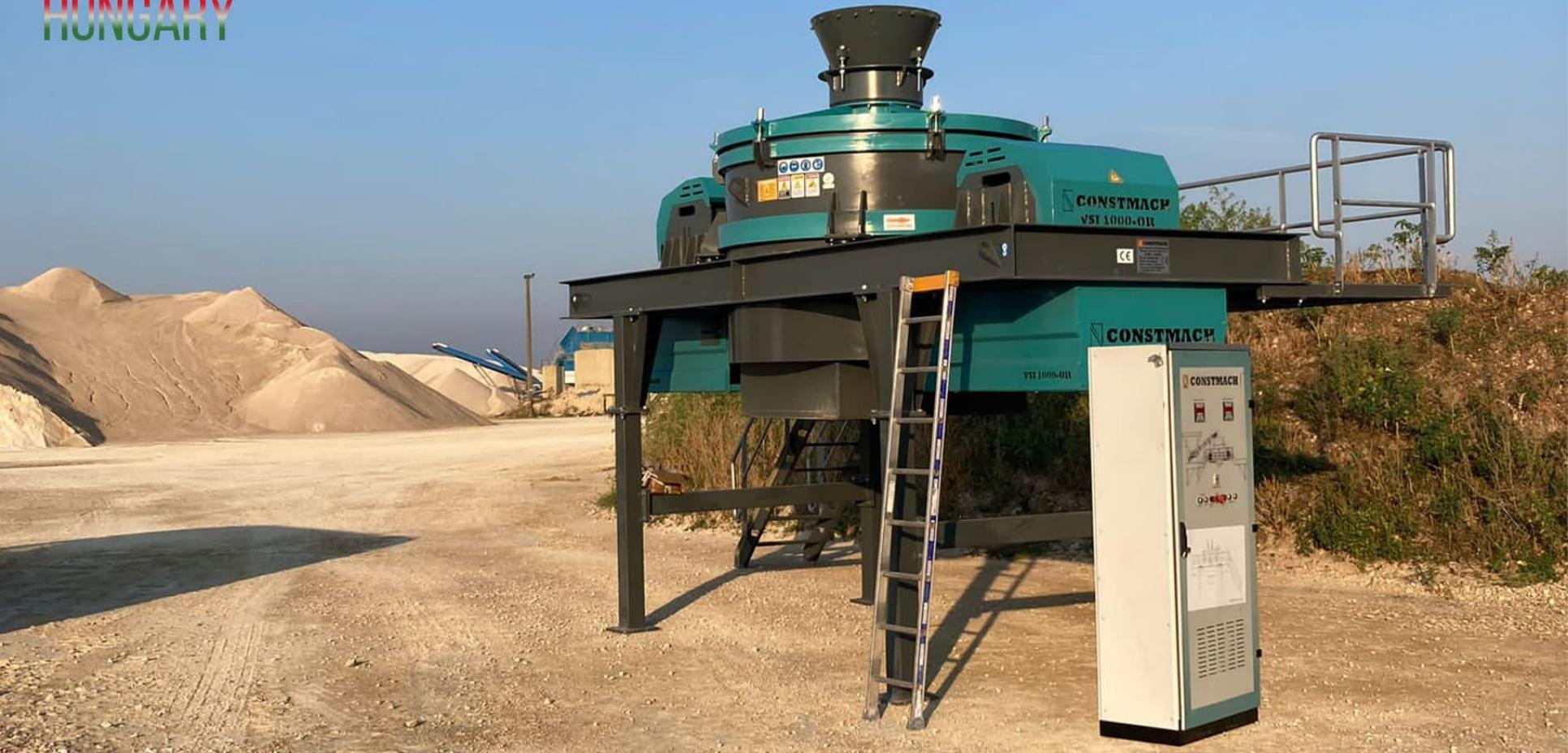
**VSI 1000 / OPEN ROTOR VERTICAL SHAFT IMPACT CRUSHER**
