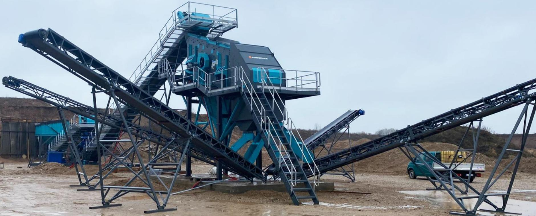
**STATIONARY CRUSHING & SCREENING & WASHING PLANT**
