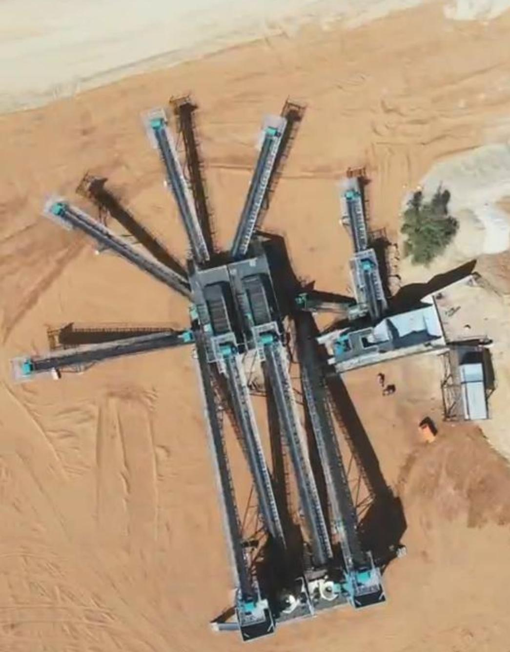
**CONSTMACH** designs and manufactures stationary crushing and screening plants with various configurations and capacity options to meet clients' needs and preferences. The production capacity of our crushing and screening plants ranges from **50 to 1,000 tons per hour**.
