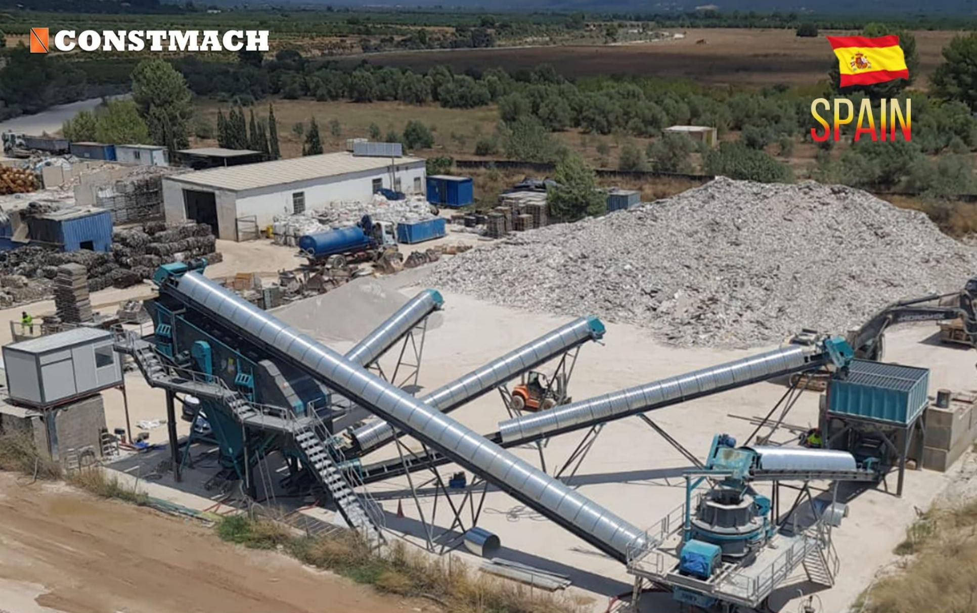
**FIX V-90 / STATIONARY CRUSHING AND SCREENING PLANT**
