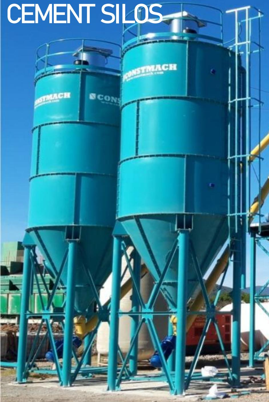
CONSTMACH manufactures different sizes and types of cement storage silos from 50 to 3.000 tons storage capacity. Cement silos are used not only in concrete plants but also they are used as an independent purposes such as cement terminals, cement factories and limestone powder stocking projects.
