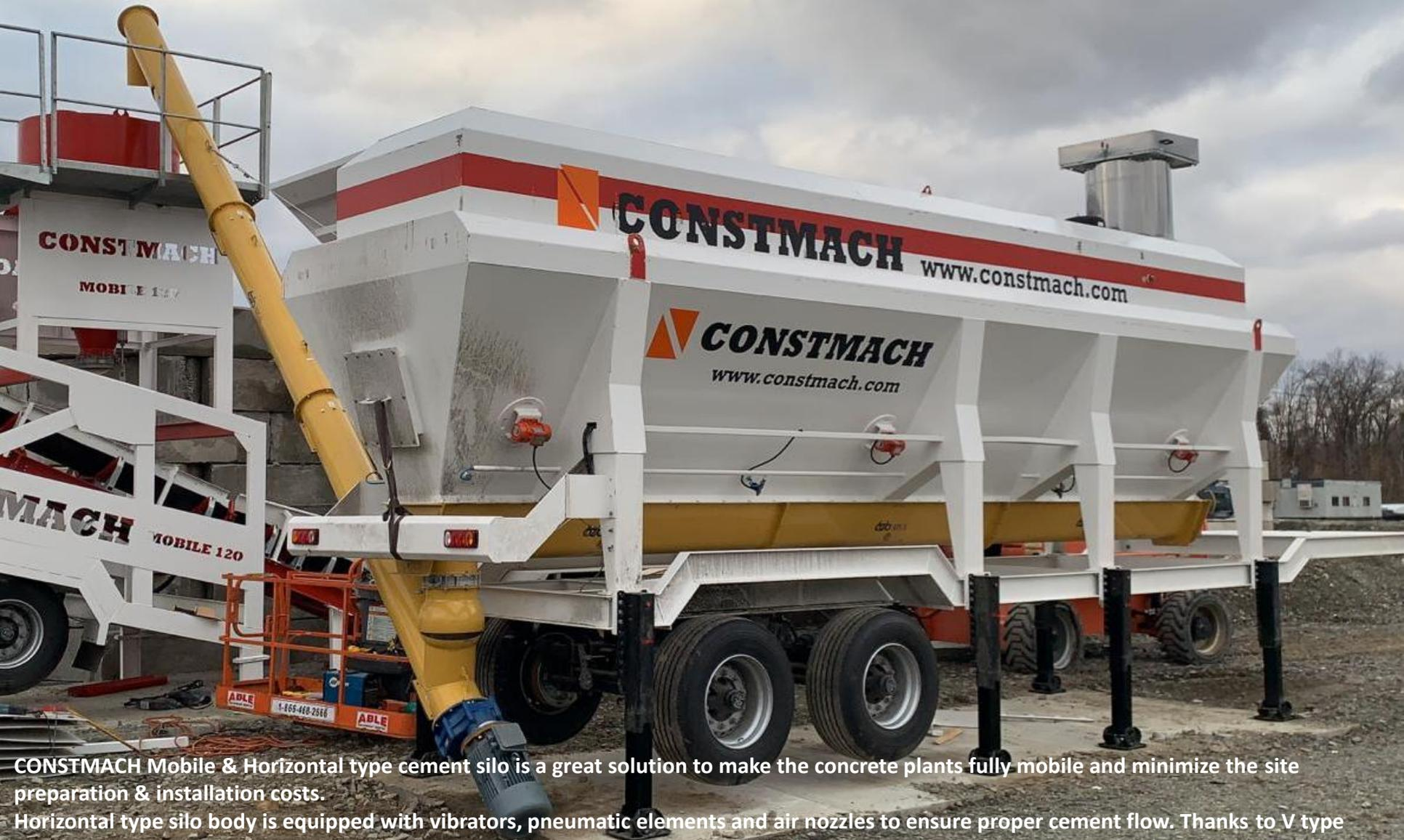
CONSTMACH Mobile & Horizontal type cement silo is a great solution to make the concrete plants fully mobile and minimize the site preparation & installation costs.
