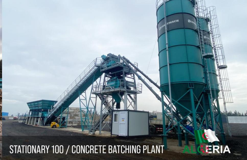
STATIONARY 100 / CONCRETE BATCHING PLANT
