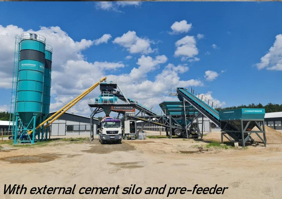
*With external cement silo and pre-feeder*
