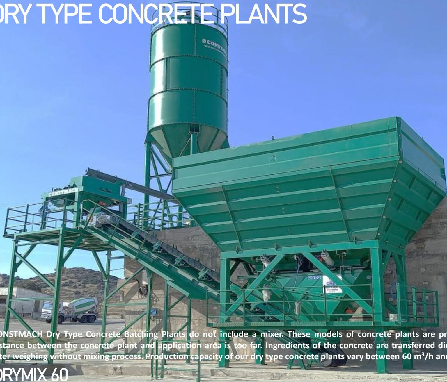
CONSTMACH Dry Type Concrete Batching Plants do not include a mixer. These models of concrete plants are preferred especially if the distance between the concrete plant and application area is too far. Ingredients of the concrete are transferred directly to the truck mixer after weighing without mixing process. Production capacity of our dry type concrete plants vary between 60 m<sup>3</sup>/h and 120 m<sup>3</sup>/h.
