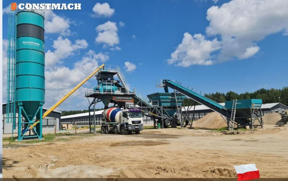
MOBILE 100 / CONCRETE BATCHING PLANT
