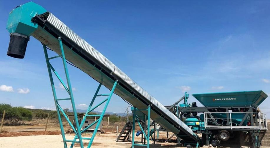
MOBICOM 30 / CONCRETE BATCHING PLANT
